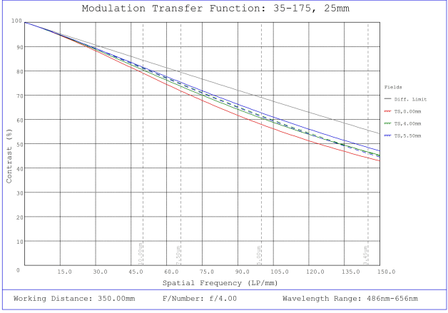
#35-175, 25mm, f/4 Cr Series Fixed Focal Length Lens, Modulated Transfer Function (MTF) Plot, 350mm Working Distance, f4
