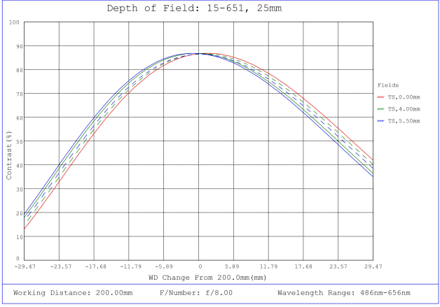
#15-651, 25mm, f/8 Cw Series Fixed Focal Length Lens, Depth of Field Plot, 200mm Working Distance, f8
