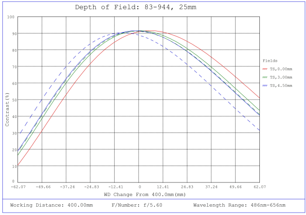
#83-944, 25mm FL f/5.6, Blue Series M12 Lens, Depth of Field Plot, 400mm Working Distance, f5.6
