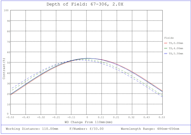
#67-306, 2X, 110mm WD, In-Line CompactTL™ Telecentric Lens, Depth of Field Plot, 110mm Working Distance, f33
