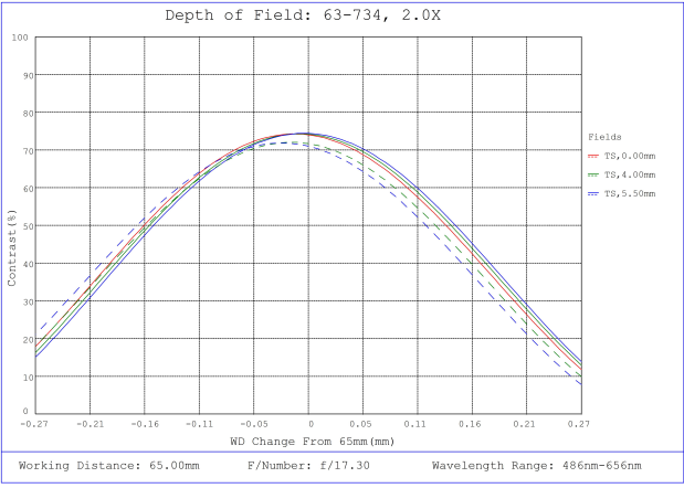
#63-734, 2X, 65mm WD CompactTL™ Telecentric Lens, Depth of Field Plot, 65mm Working Distance, f17.3
