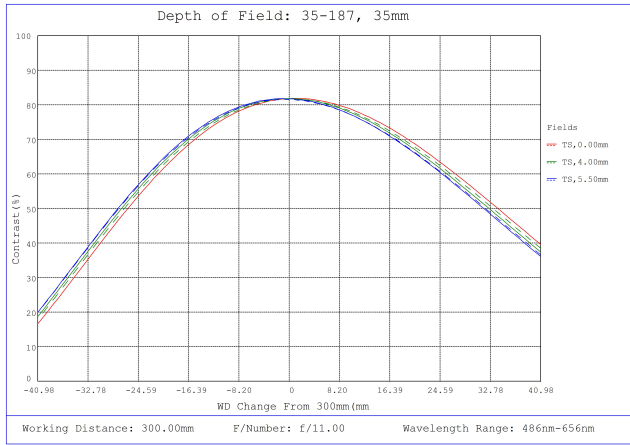
#35-187, 35mm, f/11 Cr Series Fixed Focal Length Lens, Depth of Field Plot, 300mm Working Distance, f11
