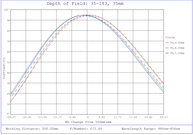
#35-183, 35mm, f/2.8 Cr Series Fixed Focal Length Lens, Depth of Field Plot, 500mm Working Distance, f2.8
