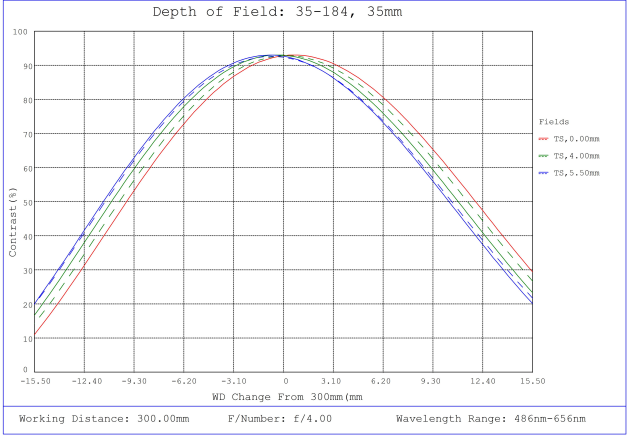
#35-184, 35mm, f/4.0 Cr Series Fixed Focal Length Lens, Depth of Field Plot, 300mm Working Distance, f4
