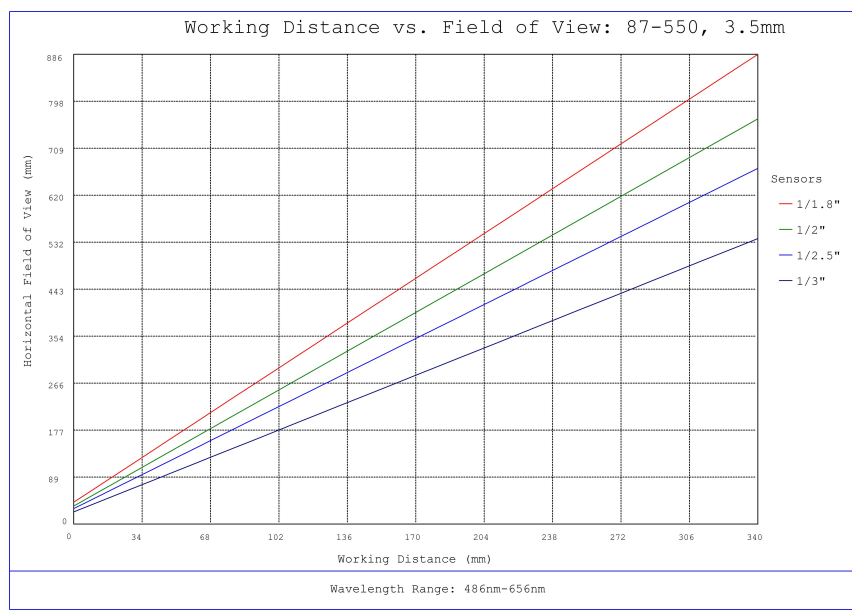
#87-550, 3.5mm, f/11 Ci Series Fixed Focal Length Lens, Working Distance versus Field of View Plot
