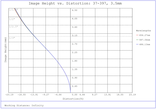
#37-397, 3.5mm, f/11 Cr Series Fixed Focal Length Lens, Distortion Plot
