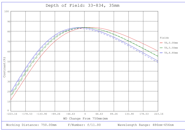
#33-834, 35mm f/11.0, HPI Series Fixed Focal Length Lens, Depth of Field Plot, 750mm Working Distance, f11
