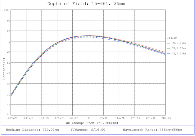
#15-661, 35mm, f/16 Cw Series Fixed Focal Length Lens, Depth of Field Plot, 750mm Working Distance, f16
