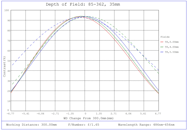
#85-362, 35mm, f/1.65 Ci Series Fixed Focal Length Lens, Depth of Field Plot, 300mm Working Distance, f1.6
