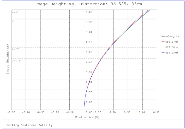
#36-525, 35mm f/1.8, HPr Series Fixed Focal Length Lens, Distortion Plot
