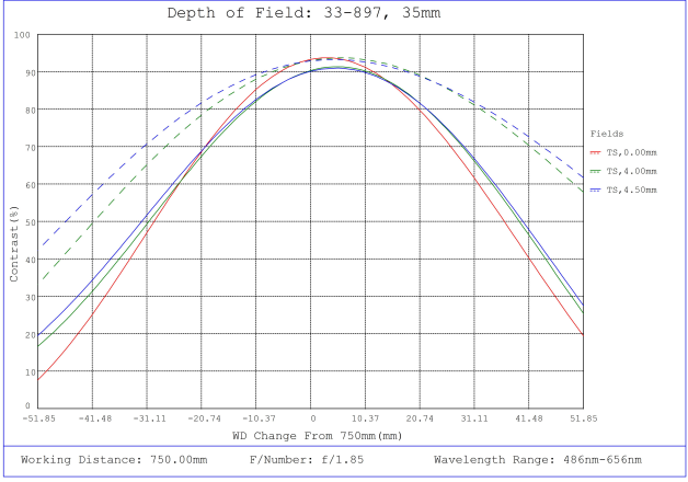
#33-897, 35mm f/1.85, UCi Series Fixed Focal Length Lens, Depth of Field Plot, 750mm Working Distance, f1.8
