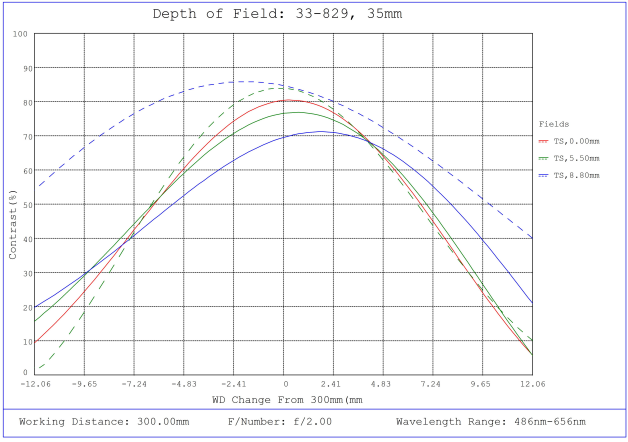
#33-829, 35mm f/2.0, HPi Series Fixed Focal Length Lens, Depth of Field Plot, 300mm Working Distance, f2
