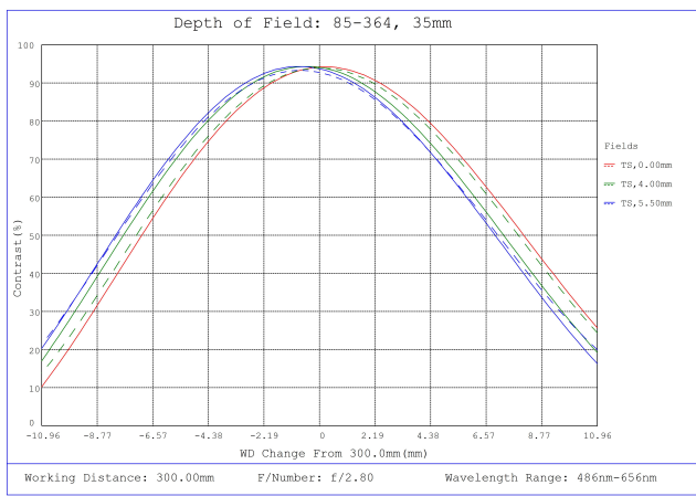
#85-364, 35mm, f/2.8 Ci Series Fixed Focal Length Lens, Depth of Field Plot, 300mm Working Distance, f2.8
