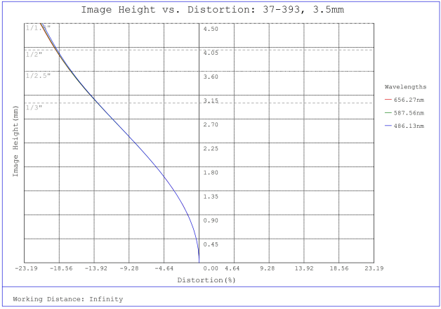
#37-393, 3.5mm, f/2.8 Cr Series Fixed Focal Length Lens, Distortion Plot
