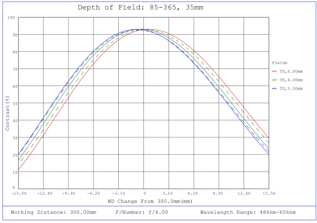
#85-365, 35mm, f/4 Ci Series Fixed Focal Length Lens, Depth of Field Plot, 300mm Working Distance, f4
