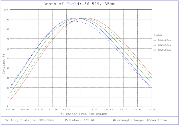
#36-529, 35mm f/5.6, HPr Series Fixed Focal Length Lens, Depth of Field Plot, 300mm Working Distance, f5.6
