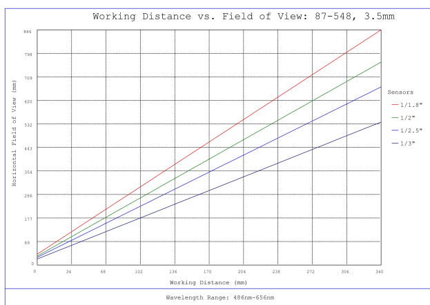
#87-548, 3.5mm, f/5.6 Ci Series Fixed Focal Length Lens, Working Distance versus Field of View Plot
