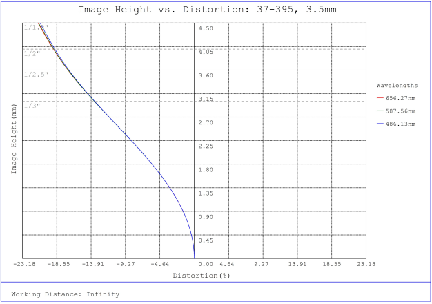
#37-395, 3.5mm, f/5.6 Cr Series Fixed Focal Length Lens, Distortion Plot
