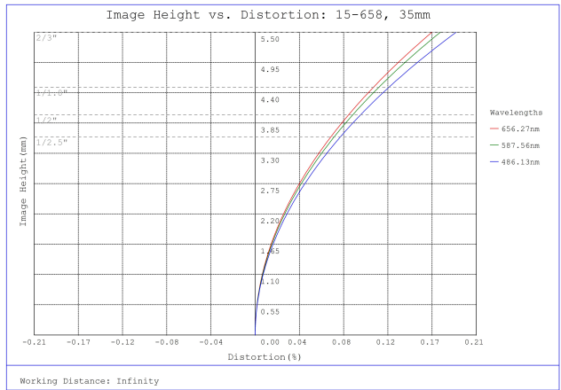
#15-658, 35mm, f/5.6 Cw Series Fixed Focal Length Lens, Distortion Plot
