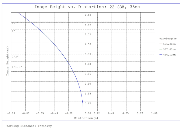
#22-838 - 35mm Focal Length, UAV Series Fixed Focal Length Lens, Distortion Plot
