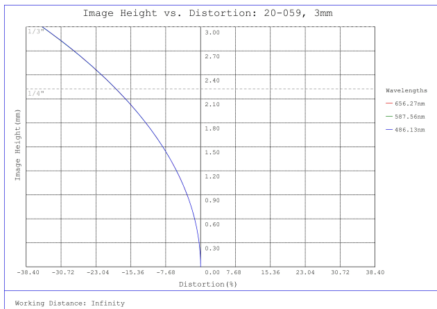
#20-059, 3mm FL f /2.5 IR-Cut Rugged Blue Series M12 Lens, Distortion Plot
