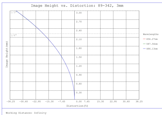
#89-342, 3mm FL f/5.6, Blue Series M12 Lens, Distortion Plot
