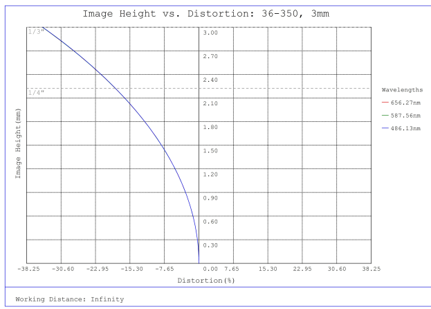
#36-350, 3mm FL f/5.6, Rugged Blue Series M12 Lens, Distortion Plot
