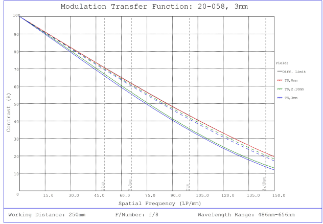
#20-058, 3mm FL f/8.0, IR-Cut Blue Series M12 Lens, Modulated Transfer Function (MTF) Plot, 250mm Working Distance, f8
