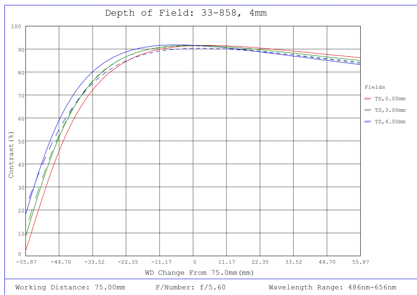
#33-858, 4mm, f/5.6 UCI Series Fixed Focal Length Lens, Depth of Field Plot, 75mm Working Distance, f5.6
