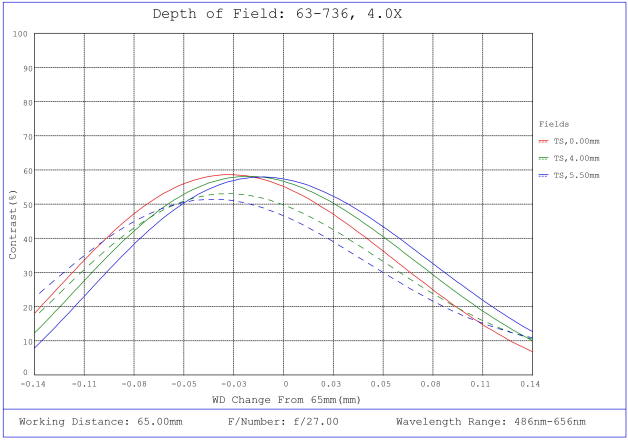
#63-736, 4X, 65mm WD CompactTL™ Telecentric Lens, Depth of Field Plot, 65mm Working Distance, f27
