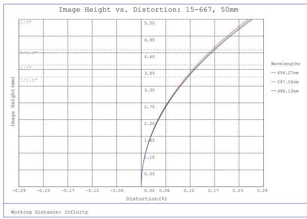
#15-667, 50mm, f/11 Sealed Cw Series Fixed Focal Length Lens, Distortion Plot
