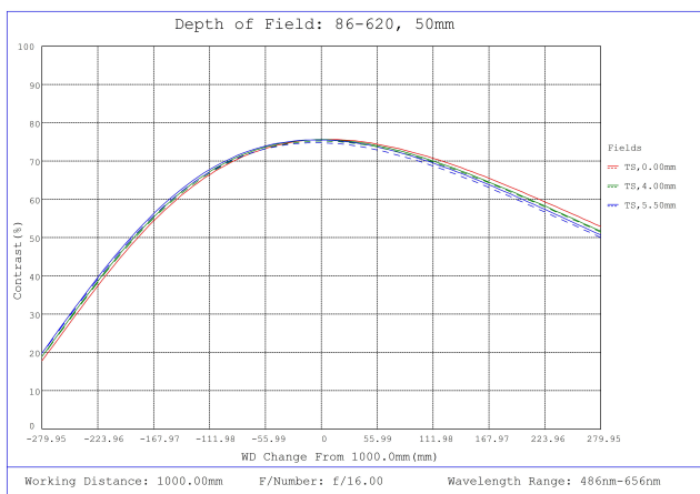
#86-620, 50mm, f/16.0 Ci Series Fixed Focal Length Lens, Depth of Field Plot, 1000mm Working Distance, f16
