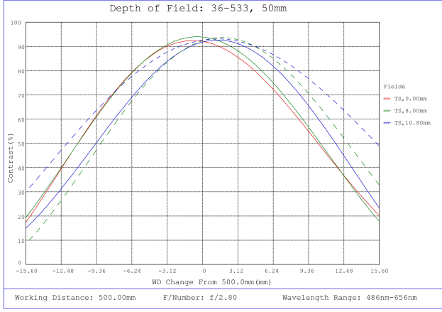
#36-533, 50mm f/2.8, HPr Series Fixed Focal Length Lens, Depth of Field Plot, 500mm Working Distance, f2.8
