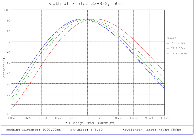
#33-838, 50mm f/5.6, HPi Series Fixed Focal Length Lens, Depth of Field Plot, 1000mm Working Distance, f5.6
