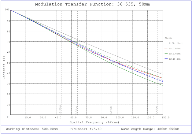
#36-535, 50mm f/5.6, HPr Series Fixed Focal Length Lens, Modulated Transfer Function (MTF) Plot, 500mm Working Distance, f5.6
