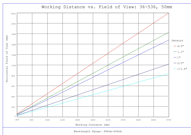
#36-536, 50mm f/8.0, HPr Series Fixed Focal Length Lens, Working Distance versus Field of View Plot
