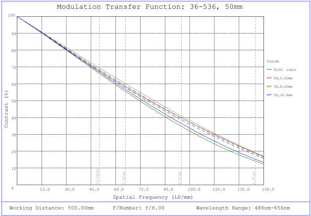
#36-536, 50mm f/8.0, HPr Series Fixed Focal Length Lens, Modulated Transfer Function (MTF) Plot, 500mm Working Distance, f8
