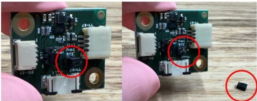
Jumper at ST2 installed
