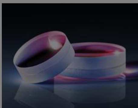
#32-313 - 12.5mm Dia. x 30mm FL, MgF 2 Coated, Achromatic Doublet Lens €86,00
