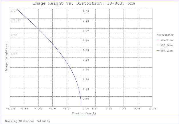
#33-863, 6mm, f/2.8 UCi Series Fixed Focal Length Lens, Distortion Plot
