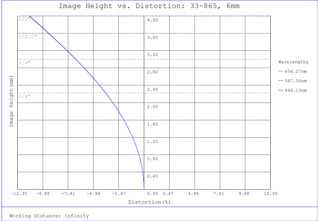
#33-865, 6mm, f/5.6 UCi Series Fixed Focal Length Lens, Distortion Plot
