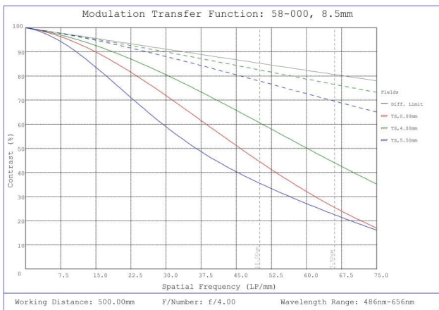
#58-000, 8.5mm C Series Fixed Focal Length Lens, Modulated Transfer Function (MTF) Plot, 500mm Working Distance, f4
