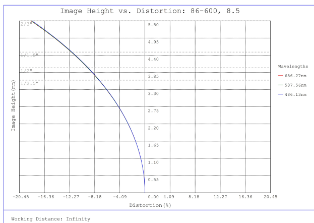
#86-600, 8.5mm, f/1.8 Ci Series Fixed Focal Length Lens, Distortion Plot
