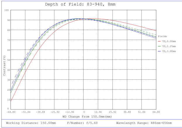
#83-940, 8mm FL f/5.6, Blue Series M12 Lens, Depth of Field Plot, 150mm Working Distance, f5.6
