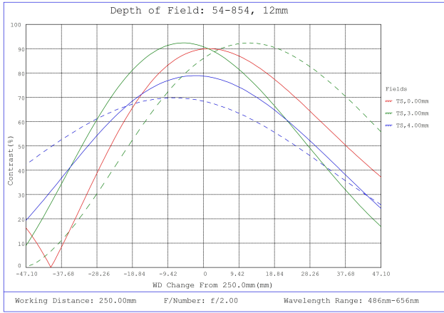
#54-854, f/2, 12mm Focal Length Green Series M12 Lens, Depth of Field Plot, 250mm Working Distance, f2
