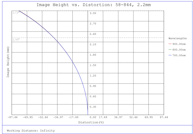
#58-844, f/2.0, NIR, 2.2mm HEO Series M12 Lens, Distortion Plot
