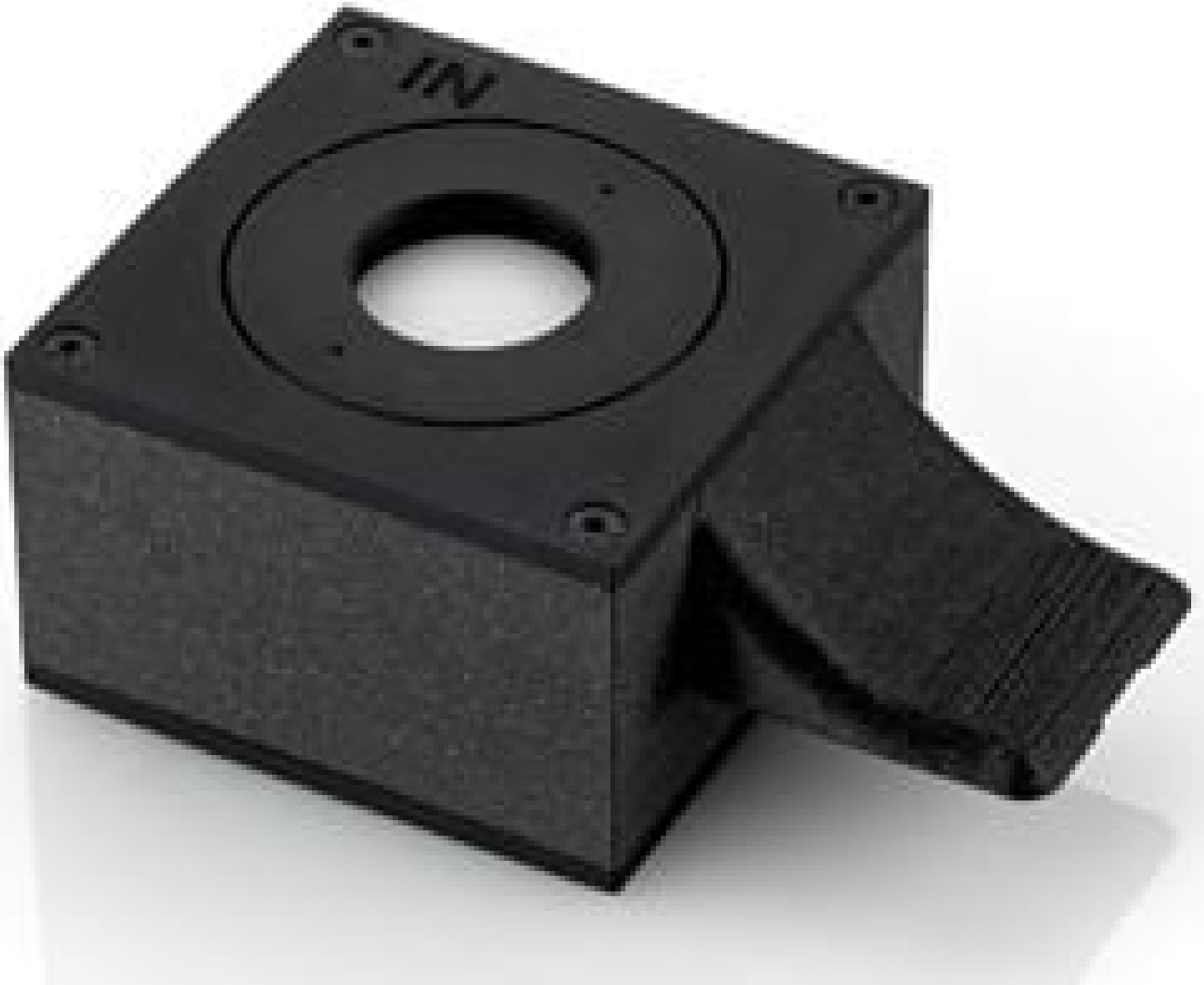
fNIRS Standard Phantom - IEC 80601-2-71
